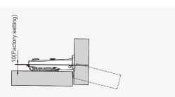
Projection of the door from the cabinet side at the max opening. The figures are based on a straight arm hinge, H=0mm mounting plate and drilling distance (K)=5mm.
