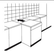
The height of the dishwasher, 845 mm, has been designed in order to allow the machine to be fitted between existing cabinets of the same height in modern fitted kitchens. The feet can be adjusted so that correct height is reached.
