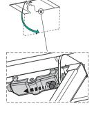
Screw the Frame into place using the 6 screws 12f, reconnect the wires to the Commands and Light, replace the metal grease filter and the Panel.
