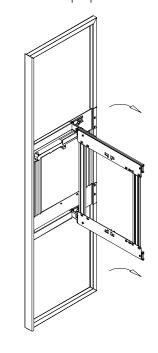
Flip unit over to mount for Left side opening.
